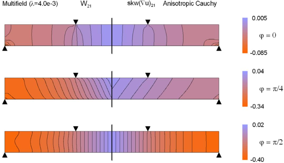
Figure 4: Contour map of the fibre rotation. On the left: multifield model ( $\lambda = 4.0 \times 10^{-3}$ ), map of the microrotation field. On the right: anisotropic Cauchy model, map of the skew-symmetric part of the displacement gradient (macrorotation).
