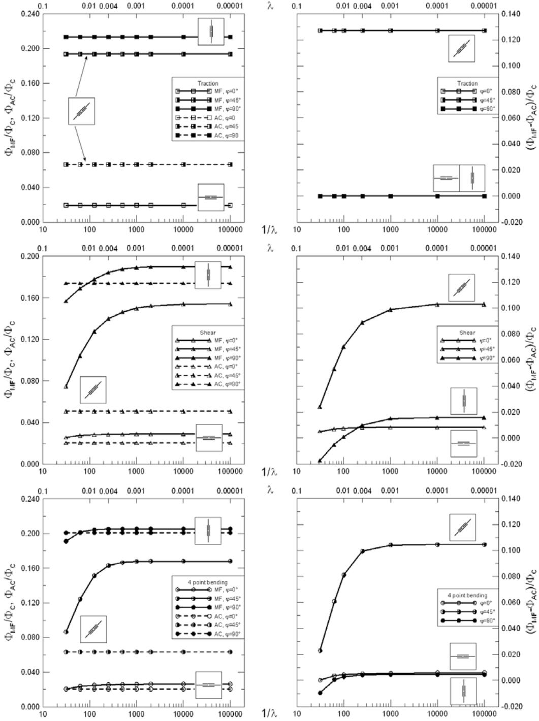
Figure 5: Deformability vs. scale factor  $\lambda$ : (a) traction; (b) shear; (c) bending. On the left: total strain energy for the multifield,  $\Phi_{MF}$ , and the anisotropic Cauchy,  $\Phi_{AC}$ , models. On the right: difference between the two models.
