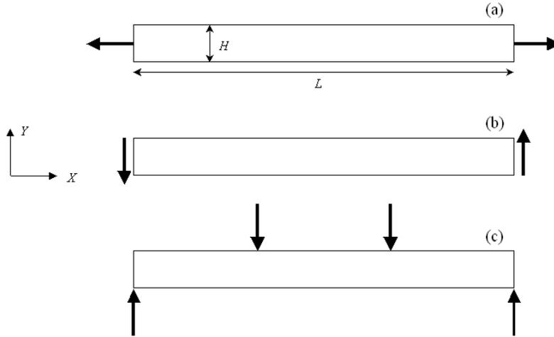
Figure 2: Sketch of the simulated system, a beam of length  $L$  and height  $H = L/10$ . Loading cases: (a) traction test; (b) shear test; (c) 4-point bending test.
