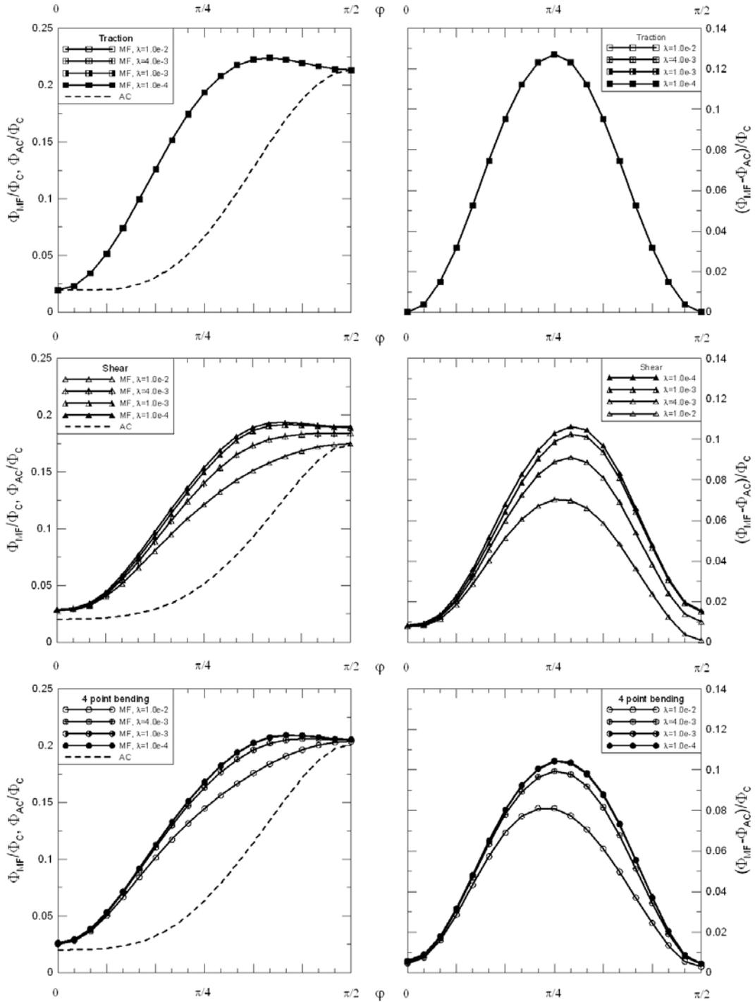
Figure 3: Deformability vs. fibre orientation  $\varphi$ : (a) traction; (b) shear; (c) bending. On the left: total strain energy for the multifield,  $\Phi_{MF}$ , and the anisotropic Cauchy,  $\Phi_{AC}$ , models. On the right: difference between the two models.
