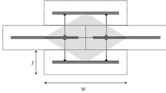
Figure 1: Sketch of the orthotropic lattice module adopted as microscopic model.
